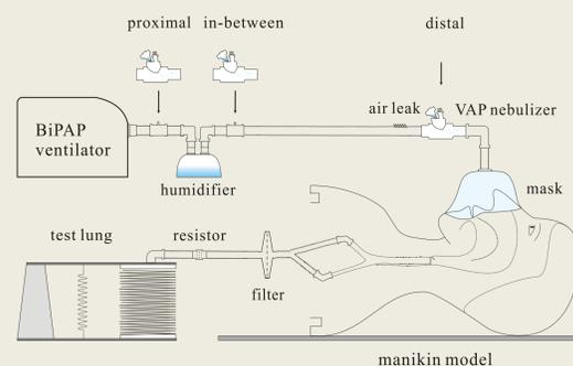
**Figure 1.** Experimental schematic of aerosol delivery during NIV.
