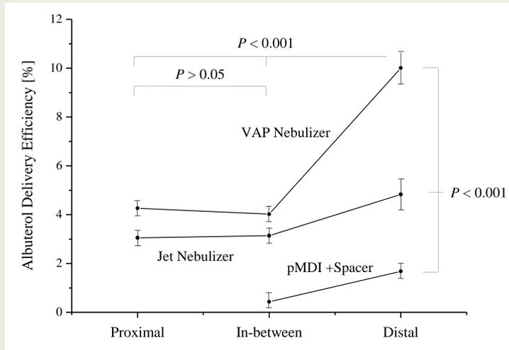
**Figure 2.** Effects of aerosol devices and their positions in the circuit on the efficiency of albuterol aerosol delivery, expressed as % of nominal dose.
