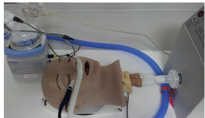
Figure 2: Respirable Dose test setup.
