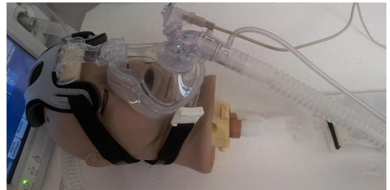
Figure 1: Respirable Dose test setup illustrating the NIVO vibrating mesh nebulizer.
