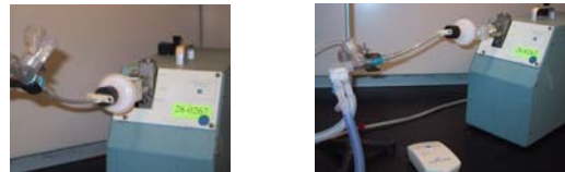
FIGURE 4: MODEL USED FOR MEASURING AEROSOL DELIVERY WITH SIMULATED INFANT BREATHING PATTERN DURING NASAL CONTINUOUS POSITIVE AIRWAY PRESSURE (nCPAP). THE PULMONARY DRUG DELIVERY SYSTEM (PDDS) PLACED ABOVE THE FILTER (LEFT) AND BELOW THE FILTER (RIGHT).
